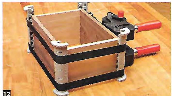
12 Rockler's box-joint-jig clamping cauls (item no. 42784, $30, rockler.com) allow you to clamp proud box joints while placing pressure squarely on the joint.
