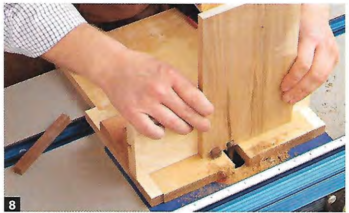
8 Fit the first socket over the pin and cut the second socket. Continue cutting, placing each newly cut socket onto the indexing pin, to complete the joint.
