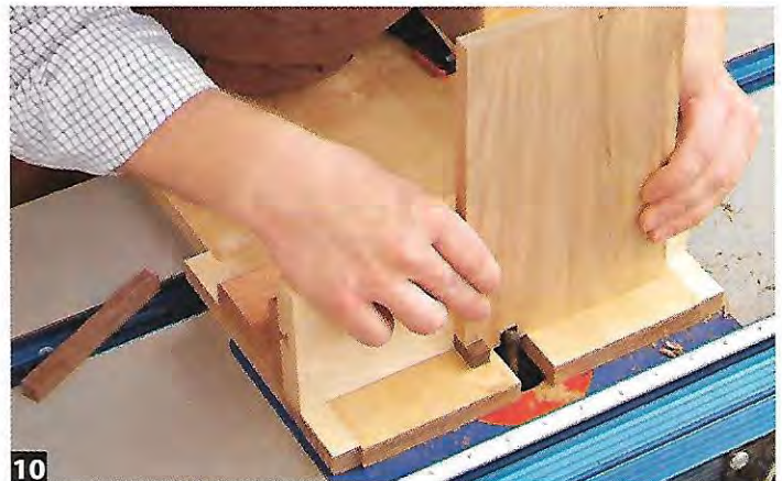
10 Fit the socket on the pin to make the next cut. Step, cut, and repeat to complete the joint. Rip the box sides to final width, trimming away partial fingers.
