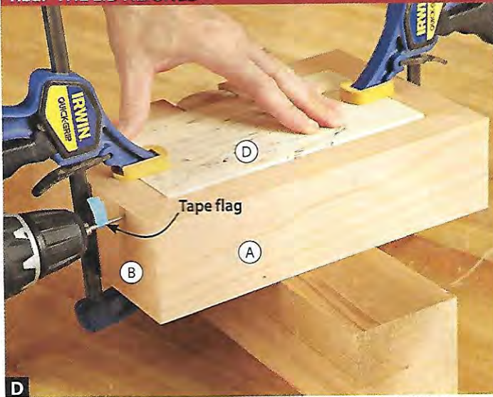
D Clamp the lid (D) in place to prevent it from shifting when you drill the holes for the hinge pins. Note the tape on the bit that serves as a depth gauge.
